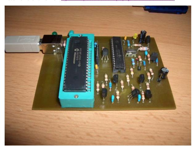
Next, the USB-Bootloader needs to be burned into the PIC. The hex file of the bootloader has been installed to your hard disc with the Microchip USB Framework installation: C:\Microchip Solutions\USB Precompiled Demos\USB Device - MCHPUSB - Bootloader 18F4550.hex
