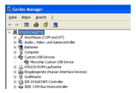
Now you start the PDFSUSB Demo application (C:\Microchip Solutions\USB Tools\Pdfsusb\PDFSUSB.exe) to burn the hex file from my homepage. Therefore select the PIC in the drop down box, open the hex file and press the "program device" button.
