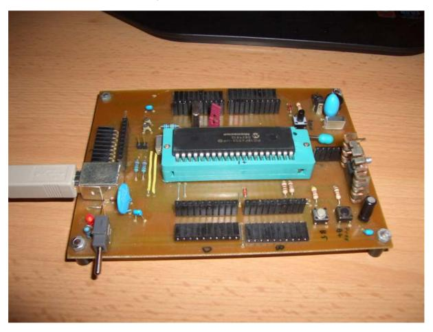
Now, to get the whole thing running, the US2BRadar firmware needs to be programmed into the PIC (hex file from my homepage). To do this, hold down the button of PORT4 (pull to ground) while pressing reset. The PIC now starts in USB boot mode.
